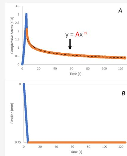
Figure 4: Stress vs Time Graph and Displacement vs Time Graph
