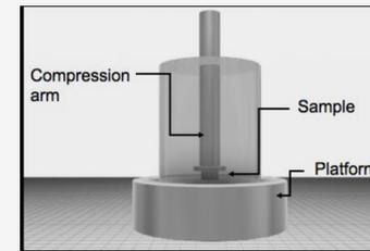
Figure 3: Model of Compression Test
